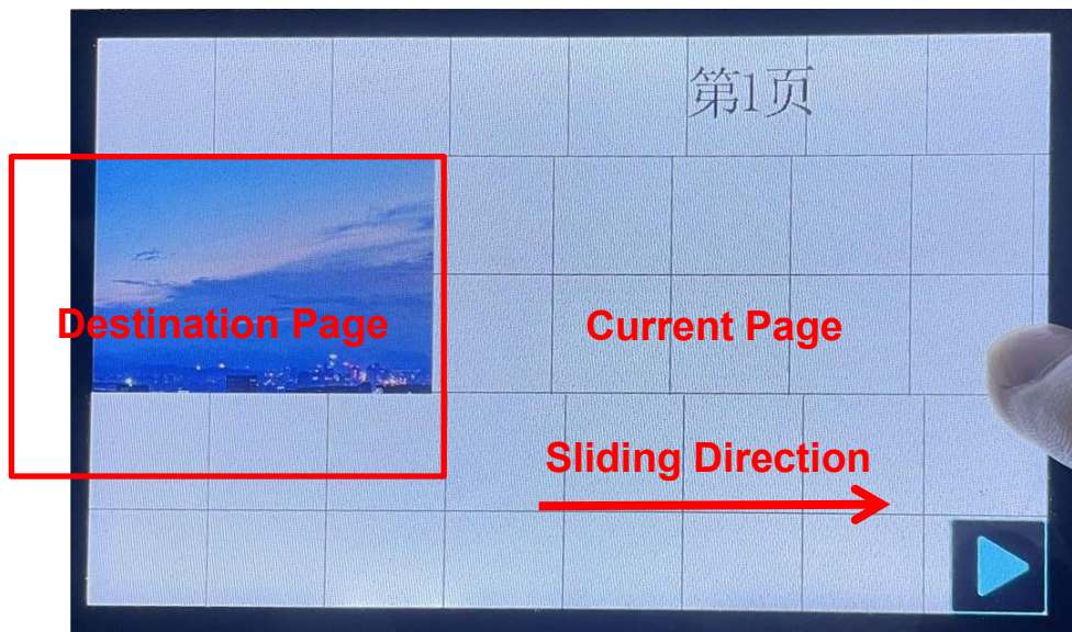
Figure 5-6: Demonstration on Sliding Area
